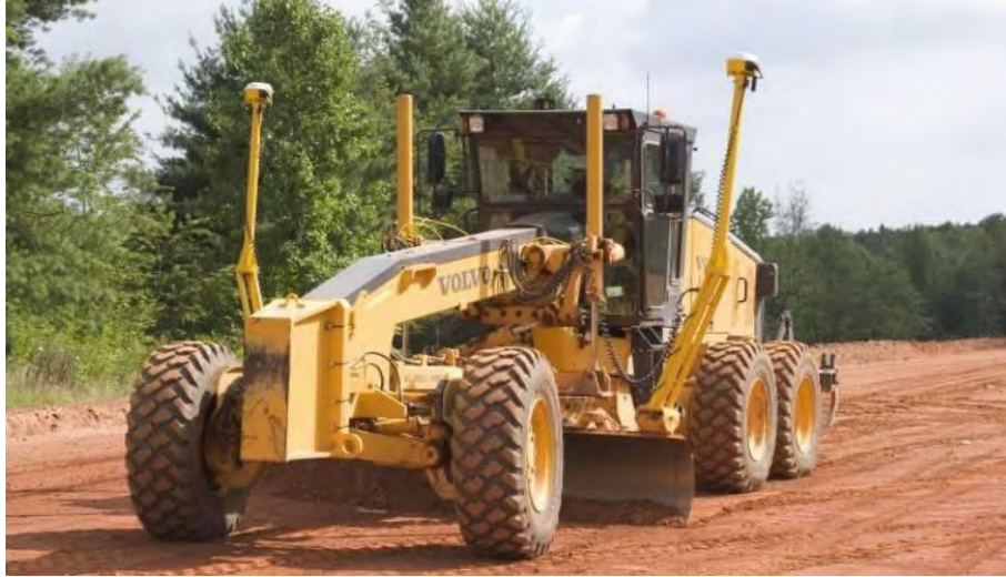
Grader equipped with AMG
