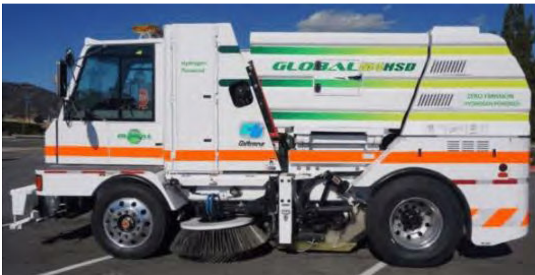
Caltrans fuel cell sweeper
